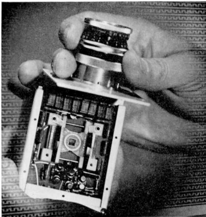
Fig. 5—The bucket-brigade camera showing the sensor.
