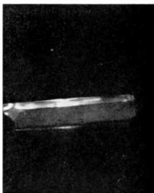
Fig. 9—Reflection from an internal heterojunction between GaP and (AlGa)P (see discussion in text).
