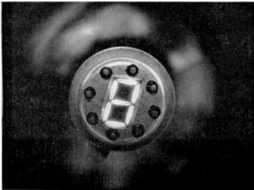
Fig. 15—Seven-segment monolithic display formed by Zn diffusion ( 4 \times 2.3 mm).
