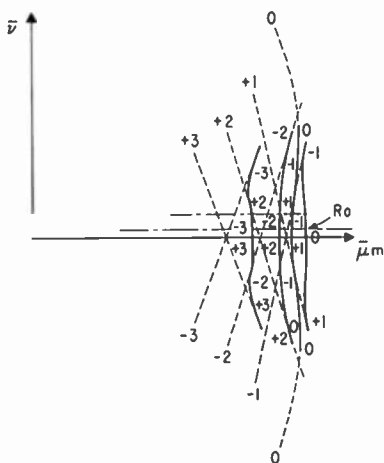
Fig. 3—Enlarged dispersion diagram near \bar{\nu} \approx 0 illustrating mode coupling at low acoustic frequencies.
