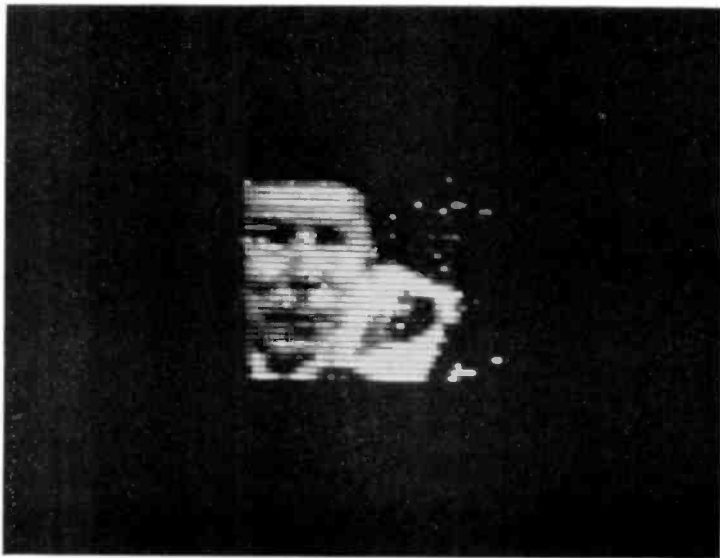
Fig. 16—A typical picture from the solid-state bucket-brigade sensor.
